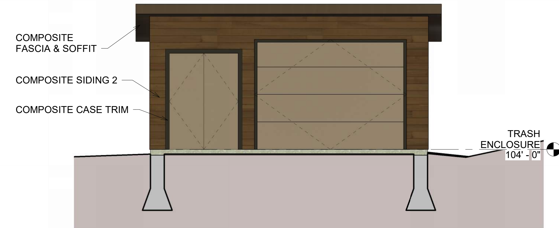
2 ELEVATION - TRASH ENCLOSURE - WEST 1/4" = 1'-0"
